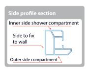
Tale the left-side profile and place it, as shown in the figure, with the widest part facing outward. Place an angle bracket marked by the number "1" in the upper part (Fig. 3.1) and an angle bracket marked by an "X" in the lower part (Fig. 3.2). IMPORTANT: The sides of the angle bracket marked by the "X" and "1" should not be inserted within the profile, but must remain outside, so that symbols remain visible.
