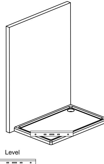
3. Remove the wall profiles, pierce 6 holes Ø6 (fig. A) and insert the 6 anchors (vedi fig. B)
