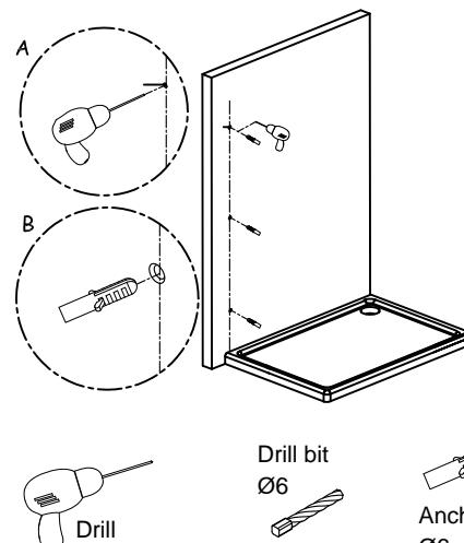
2. Place against the wall the profiles in the indicated positions, ensure they are perfectly vertical with the level and mark the positions.
