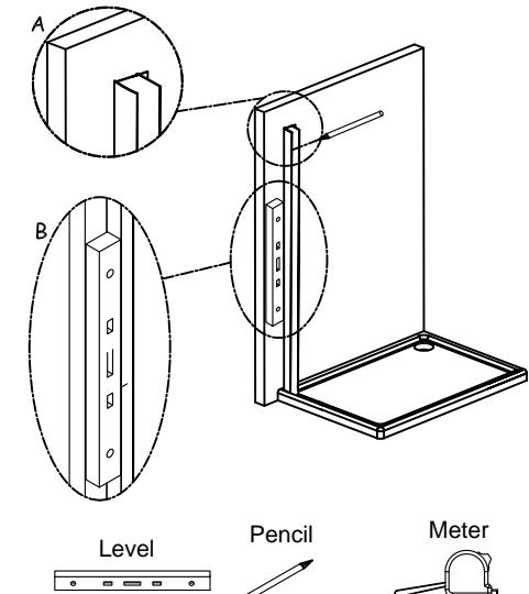
4. Installing fix side panel: insert the glass into the wall profile, secure it, and insert the corner profile on the other side.
