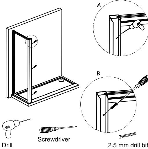
6. adjust the position of the shower enclosure, drill where prepared in order to secure the corner profile with the upright of the fixed panel, by using ST3.5\*10 screws.
