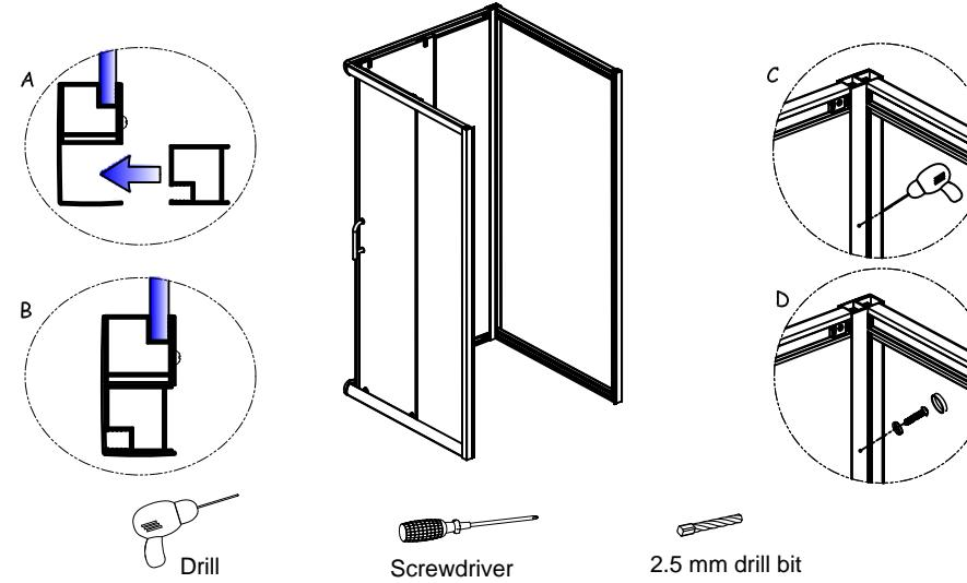
7. a. drill profiles with the wall profile with drill bit of 2.5 mm where prepared.
