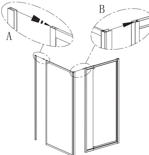
4. According to the corner profile position, drill 3 mm holes in designated positions then fasten the profile to fix panel using the ST3.9\*12 screws.
