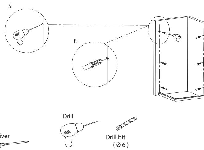
7. According to the holes positions, fasten the corner profile with ST3.9\*32 screws.
