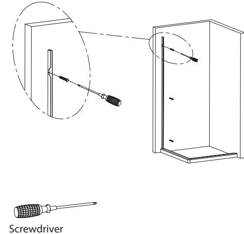
8. Place the enclosure on the wall, according to the corner profile holes, drill a 3 mm hole on wall profile ( fig. A ) then fasten it with ST3.9\*12 screw and cover ( fig. B ).
