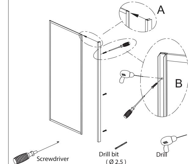
3. Like fig. A, install the fix side panel and insert the corner profile (fig. B) on opposite side.
