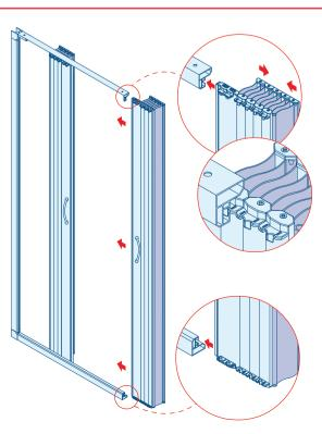
Slide the right folding door in both upper and lower rail profile, as shown in figure, making sure that all door supports are inserted in the rail profile. To make the operation easier cluster the folding doors.
