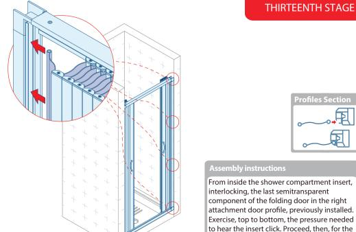
From inside the shower compartment insert, interlocking, the last semitransparent component of the folding door in the right attachment door profile, previously installed. Exercise, top to bottom, the pressure needed to hear the insert click. Proceed, then, for the entire length of the side profile.
