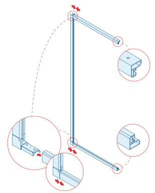
Insert the upper and lower rail profile in the angle brackets of the previously assembled left side profile.
